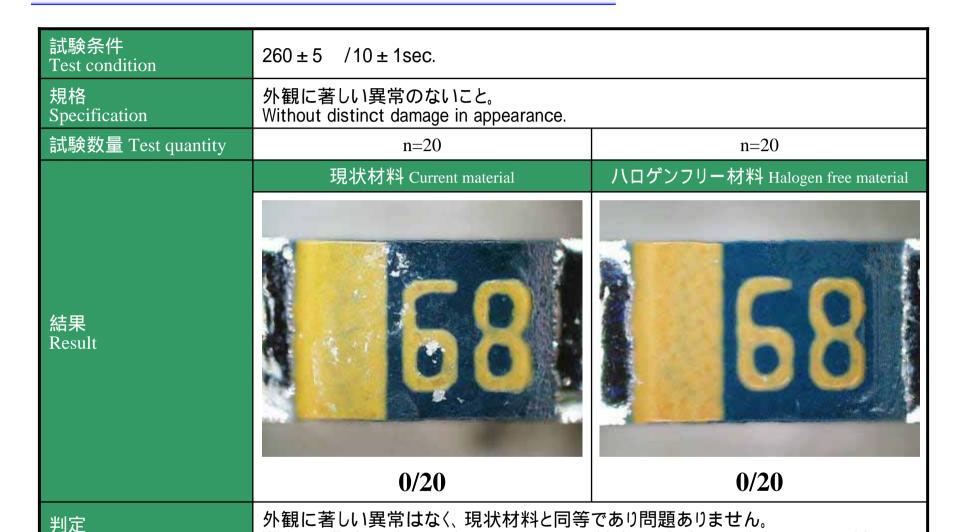
Without distinct damage in appearance, and it is equivalent and there no problem with a current material.
